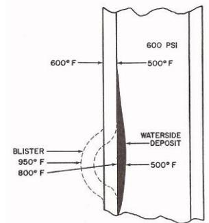
*Effects of Waterside Deposits on Boiler Tubes*
