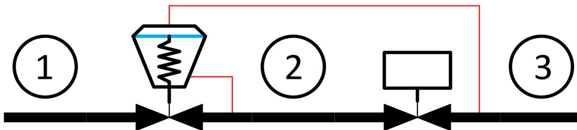
Figure 4 - PICV Conceptual Diagram
