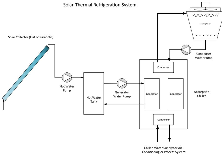
Figure 2.2 – Solar-Thermal Refrigeration System
