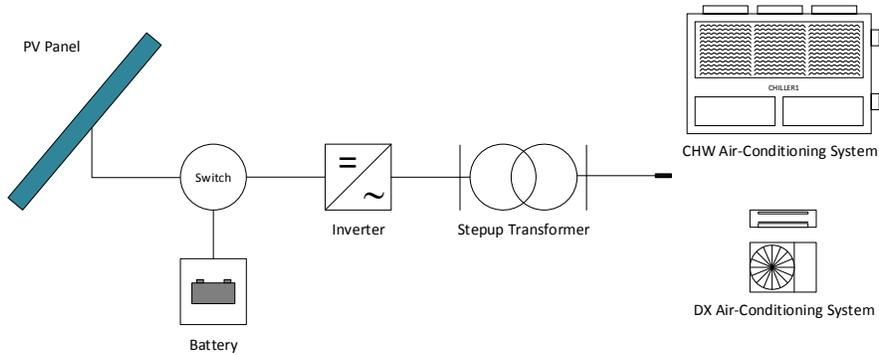
Figure 2.1 – Solar-Electric Refrigeration System
