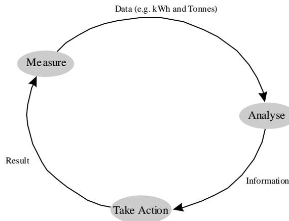
Figure - A Model of the Monitoring and Targeting Routine
